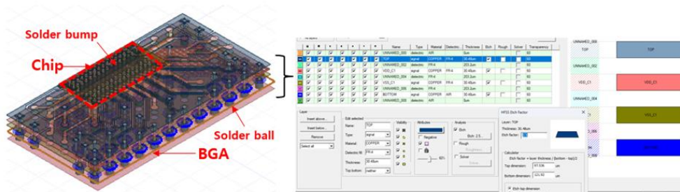
Figure 28. PCB/PKG CAD file Import, Structure and Stack-up parameters assign
