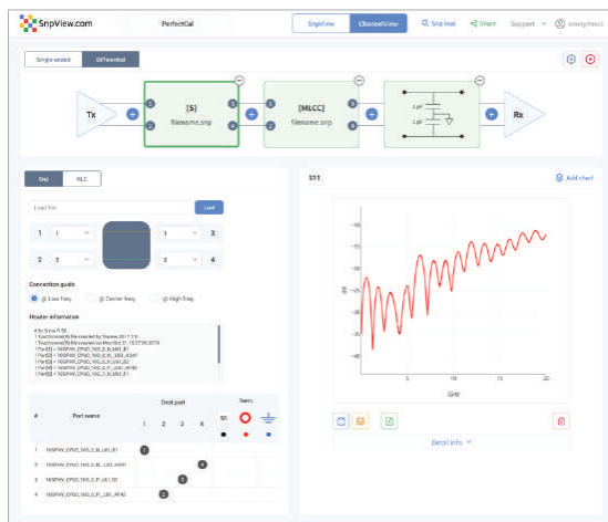
ChannelView : High-speed channel simulator with EQ/Jitter : Support PAM4 simulation
