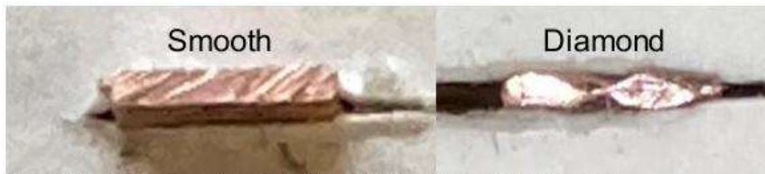
Figure 4: Conductor cross sections for the Smooth (left) and Diamond (right) conductors.
