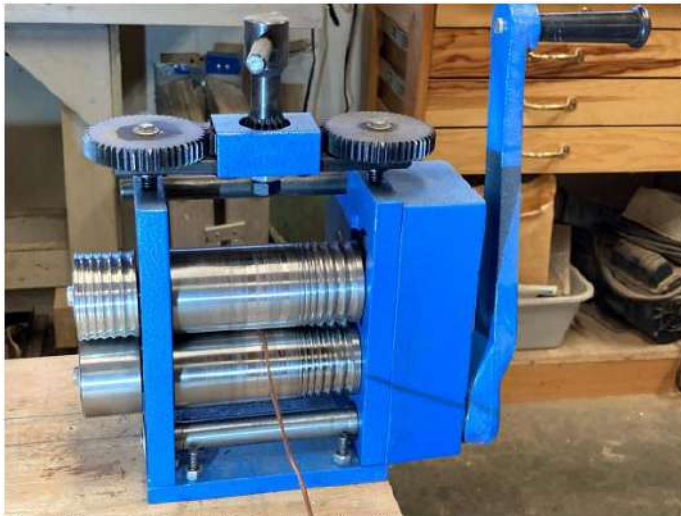
Figure 1: Copper wire being rolled in a jeweler's rolling mill.
