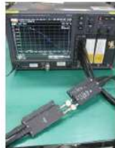
Figure 3. differential return loss measurement of TTCs using Keysight N1055A 50GHz TDR
