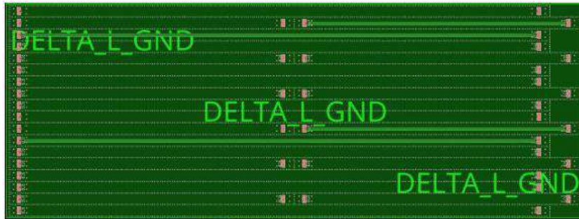
Figure 2: Delta-L Differential Pair Layout
